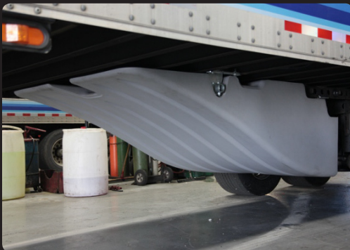
Trailers equipped with this front tray fairing can achieve between 7 and 12 percent improvements in fuel mileage. (Photo courtesy of BMI SmartTruck)
